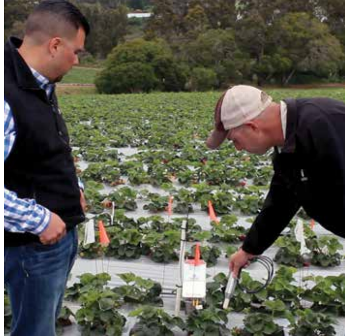
Project WIN uses probes to gauge field soil tension, sending real-time diagnostics to network base stations. Growers monitor results through wireless handheld devices.
